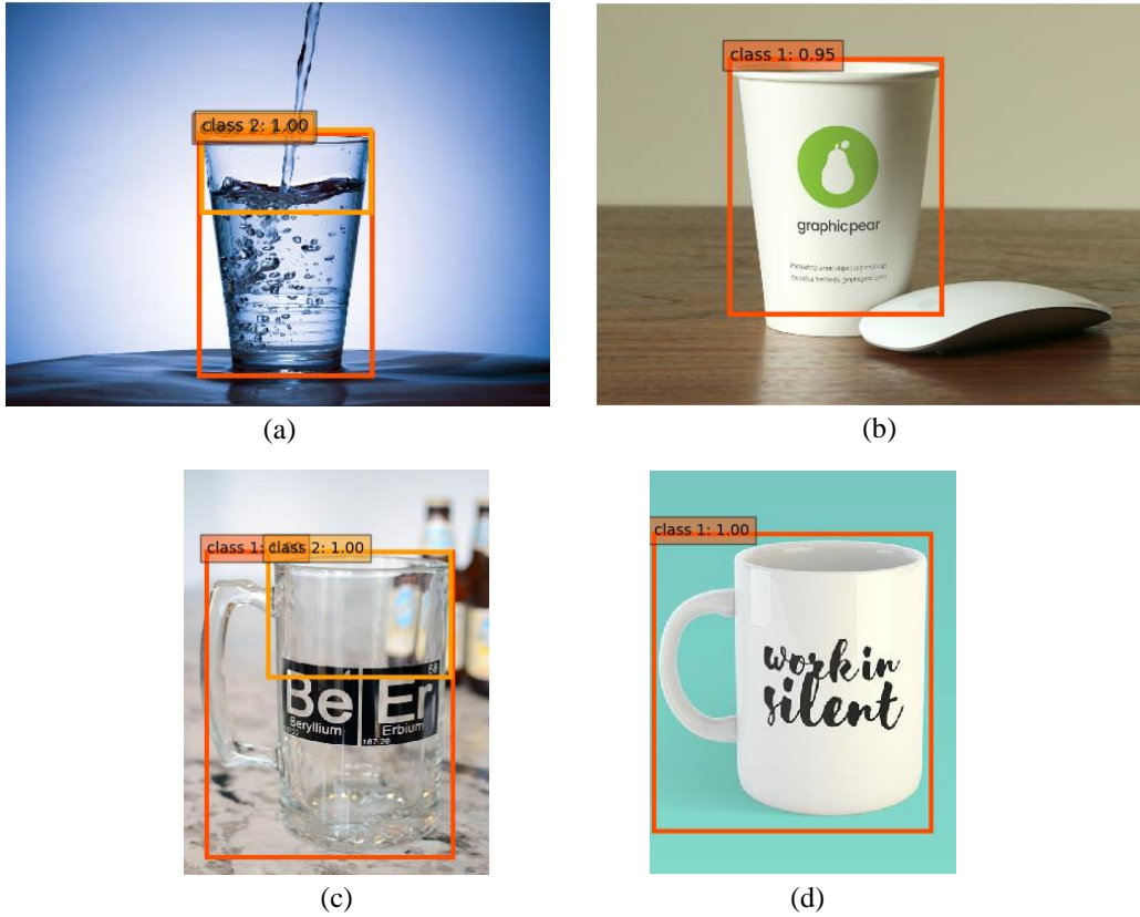
Figure 13. The detection result after training the network with glass and glass-feature region data. The label class 1 represents the glass and class 2 represents the glass-feature.
